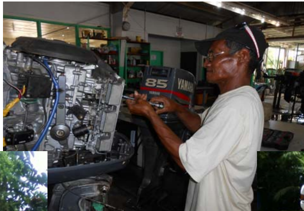
PAN Rangers troubleshoot Outboard Marine Engine
